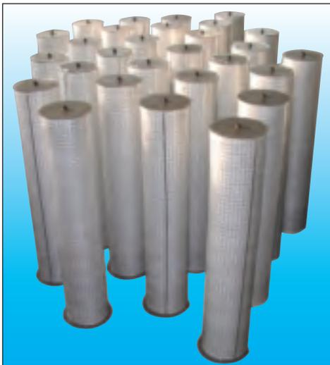
A coalescing filter is a special fiber bed into which enters a gas carrying mists and out of which gets out a clean gas and a separated condensate liquid.
